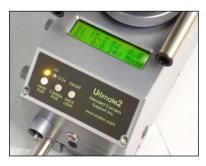
LCD screen displays total voltage into the system and current voltage remaining of each battery pack in 12 volt mode. Combined voltage in 24 volt mode.
